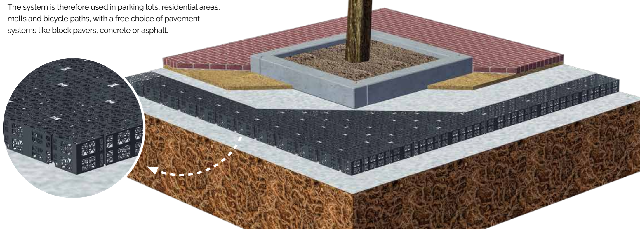
Permavoid Sandwich Construction used in a streetscape with newly designed and created elevated soil levels in the village of Geldrop, The Netherlands.
